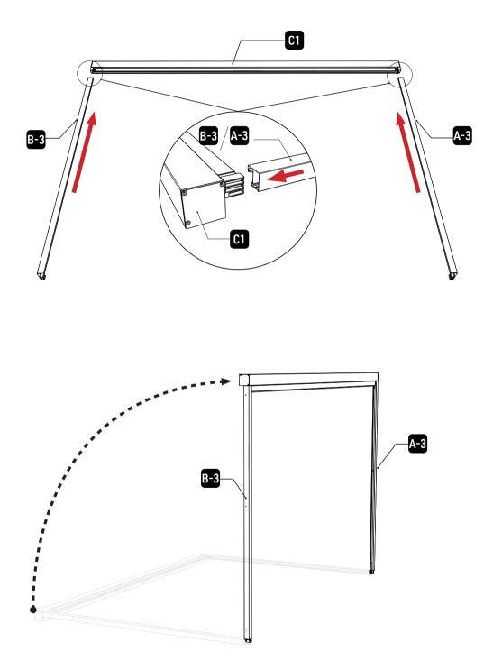
Put the frame up and make sure the outer face of wind screen box align with outer face of beam.
