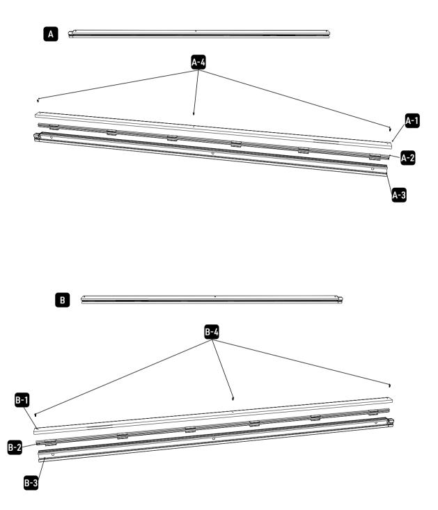
Insert A-3/B-3 into the side panel of wind screen box (C1).
