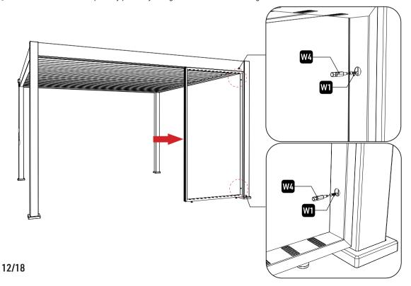
Fix the upper frame of the privacy panel by using screws(**W1**) as the diagram shows below.
