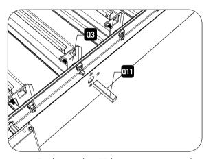
1. Place **Q11** (cylinder) on **Q3** (master louver end cap)
