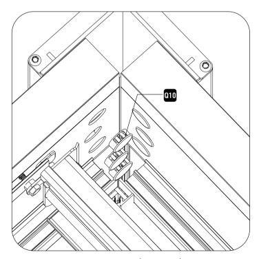
Cover holes in each corner on Beams  ${\it C/B/B1}$  with  ${\it Q10}$  (plastic cap).
