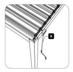
1. Remove **Q9** (box cover), place **Q9/Q8** onto **Q11** and secure with **Q21** screws. Install H into **Q8** and tighten.
