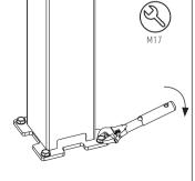
Check all dimensions of the pergola, then anchor base plate  $\mathbf{Q2}$  to concrete foundation using  $\mathbf{Q15}$  (expansion bolt). Caution the post skirting can scratch post.
