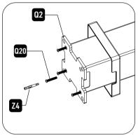
2. Use  $\bf Q20$  (socket screw 6x35) to install  $\bf Q2$  (base plate) to attach  $\bf A$  (post). Use  $\bf Z4$  (4mm bit ) to secure.
