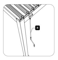
2. Remove Q9 (box cover), place Q9/Q8 onto Q11 and secure with Q21 screws. Install H into Q8 and tighten.
