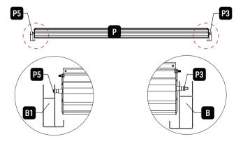
2. Insert **P3** end of Master Louver **P** first into and hole of Beam **B**. Then insert opposite side into Beam **B1**.
