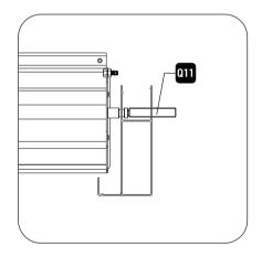
1. Place Q11 (cylinder) on P3 (master louver end cap)
