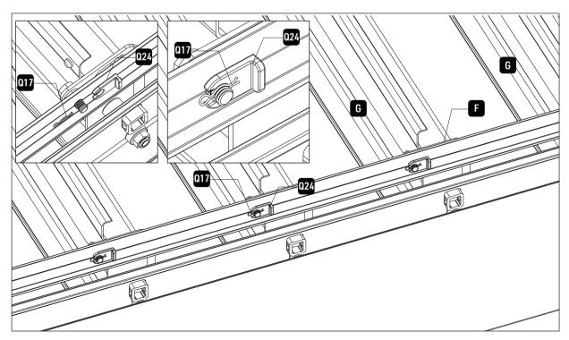
3. Place Q17 onto screw of louver end cap then insert Q24 into screw of other louver end cap. Repeat this with all louver end caps to connect F to each louver P.
