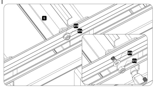
2. Place washer **Q18** onto screw of louver end cap then insert **Q16** into screw of MAIN louver end cap. Repeat this with all louver end caps to connect **F** to each louver **G**.
