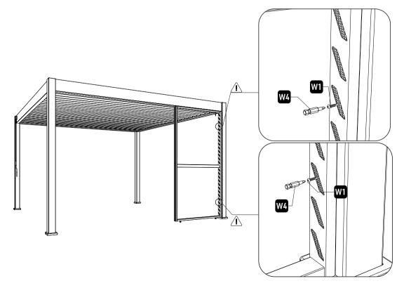
Fix the upper frame of the privacy panel by using screws(W1), then cover the hole with plastic caps(W3).
