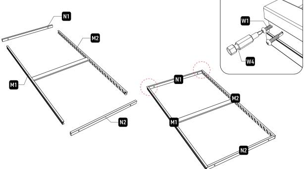
Install the adjustable base under the bottom frame , please note that do not screw the adjustable base too tight.
