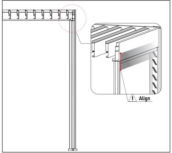
Adjust the adjustable bases again to make sure they just stand on the ground.
