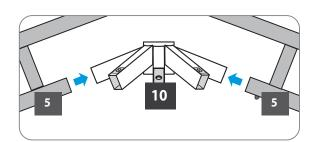
ATTENTION: The tunnels of top gable connector (10) are marked, in order to avoid mistakes when inserting the roof gable profiles.
