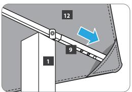
To finish stretching the canopy, press the push button in extension profile (6A) and extend extension profile (9) as far as possible to the outside until the push button snaps into place.
