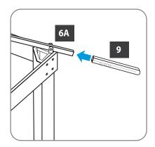
NOTE: You will need to extend profile(9) outwards to stretch the roof canopy into its final position.
