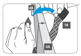
Attach roof connectors (16) to each roof profile (4A) through hole in wicker strap, as shown, using bolts (14).
