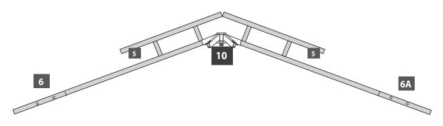
Using at least two people, connect the two roof gable profiles (5,6) and (5,6A) to roof connectors (16) on opposite corner profiles (1). Fasten with bolts (17,15) as shown.
