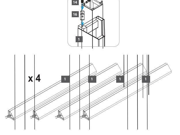
Slide support frames (2) over lower end of corner profiles(1).
