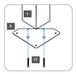
Leave support frames (2) about 10" over lower end of corner profiles (1) until step 4.
